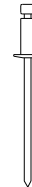
Pop Rivet Used For: -Trim Lap -Downspout to Gutter -Outside Corner Box -Downspout Strap
